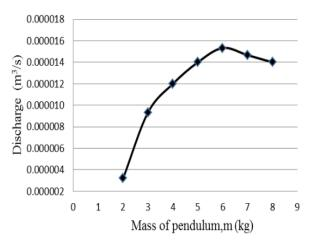
Graph 1 Mass of pendulum, (m) vs Discharge
